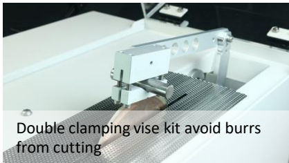
Round vise kit is designed for round samples or mounted samples
